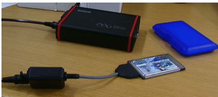
Figure 5.6: The DSP card connected to a BOSCH DAB core receiver
